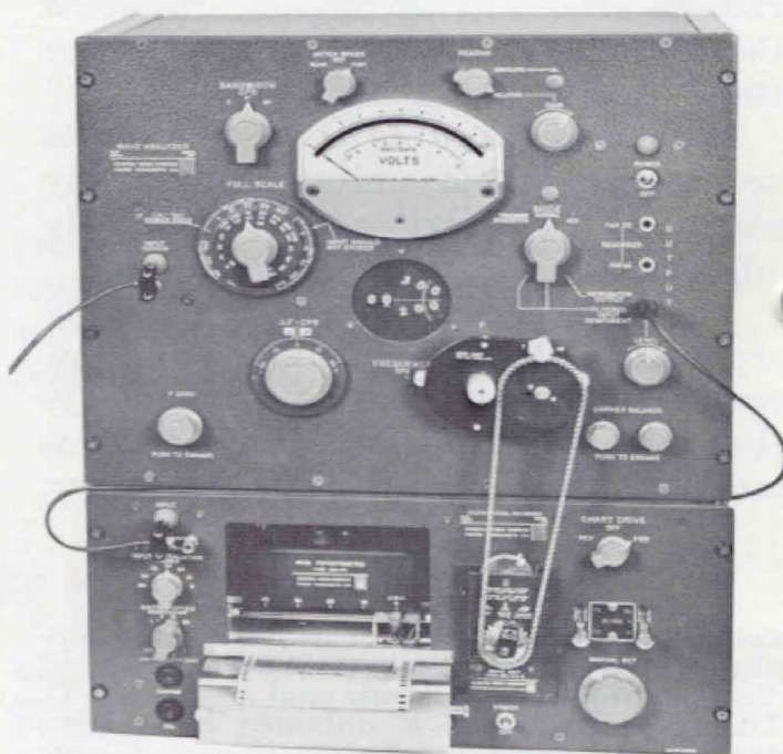
Figure 1. Type 1900-P3 Link Unit installed on the wave analyzer and graphic level recorder.
